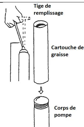
**TOUJOURS ENLEVER LA CARTOUCHE POUR REMPLIR PAR APPAREIL A POMPE, MANUELLEMENT OU PAR ASPIRATION****Remplissage par appareil**
